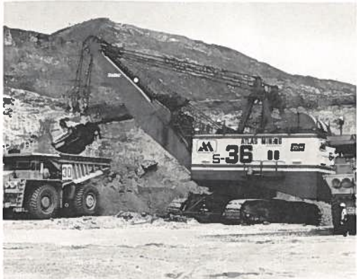
Loading operations at Biga Pit with an 18-cubic meter 201 M Marion electric shovel.
