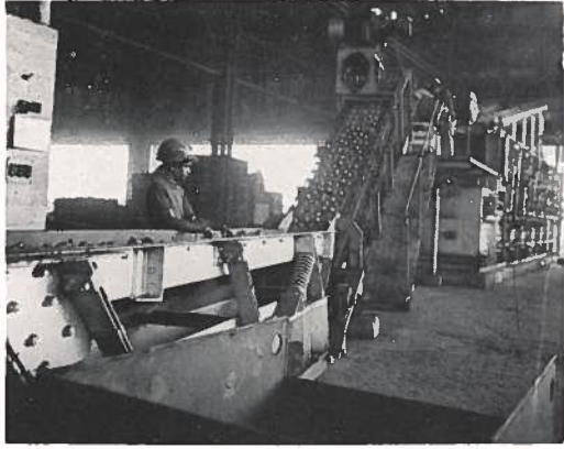
Holcroft continuous heat treatment furnace for steel balls.
