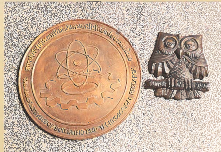
Metal casting by vacuum process moulding technique.
