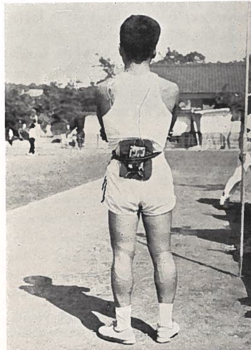
Fig. 21. A part of wireless telemeter attached to a subject. (Coutesy, Dr. Hideji Matsui)
