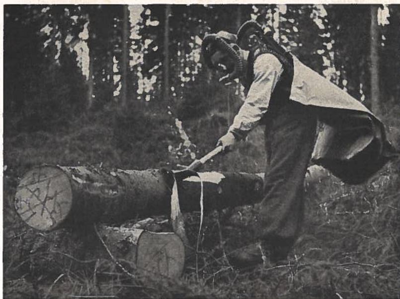
Fig. 2. Estimation of the energy output at barking with help of Douglas' bag method.
