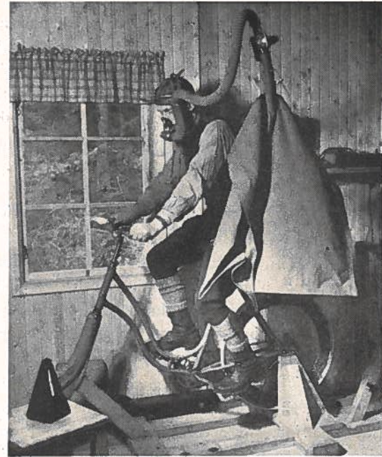
Fig. 19. A lumber man's capacity for work is tested on a bicycle ergometer.
