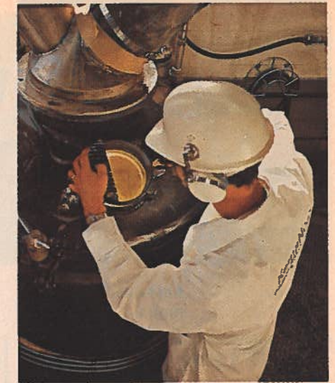
The dangerous vinyl chloride is changed – polymerized – into polyvinylchloride, which is harmless, in this big container.
