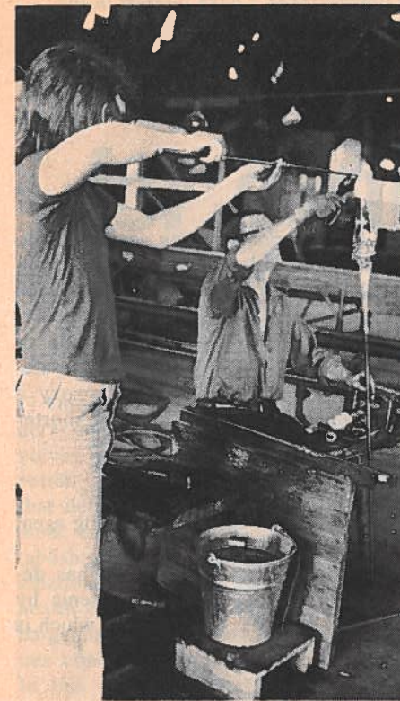
Per Olofsson helps Karl Gustav Svensson, the leg maker, attach a leg to the glass vase.
