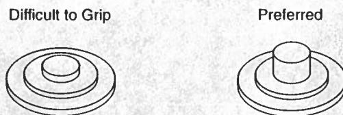
Figure 17.7 Improve parts handling by making parts easy to grip
