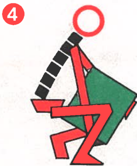
4 Use body weight to start load moving — then lift by pushing up with legs
