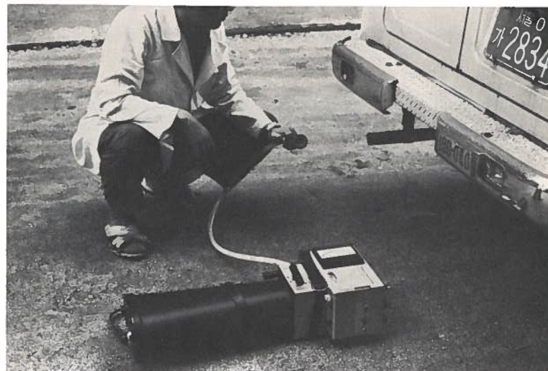
Variable filter infrared analyzer for air pollution measurement
